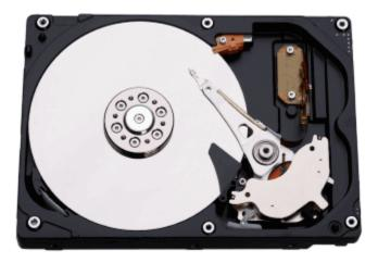
Its main components include a read/write actuator arm, head actuator, read/write head, spindle, and platter. A circuit board (also called as the interface board or disk controller) is present on the back of a hard drive. It lets the hard drive to communicate with the computer.
